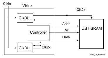
Figure 4: Virtex device and ZBT SRAM
