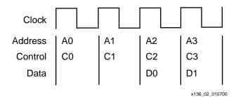
Figure 2: Bus Operations for Pipelined ZBT SRAM
