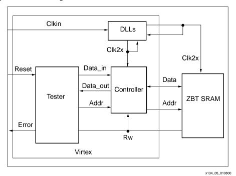
Figure 5: Block Diagram of the Verilog Design
