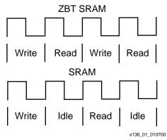
Figure 1: ZBT SRAM vs. Regular SRAM
