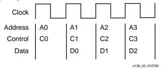
Figure 3: Bus Operations for Flowthrough ZBT SRAM
